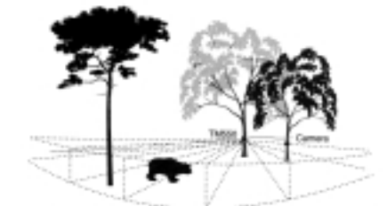
The TM550 must be mounted on a tree or post that does not move. The sensor is a heat-and-motion sensor and is dependent on being stationary to work properly. The camera can be located up to 25 feet away from the TM550.
