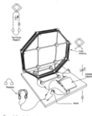
Diagram for low-budget xtal set using foil-lined paper protectors.
