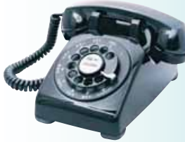
Western Electric 500 Few households of the 1950s and 1960s were without a Western Electric 500, the mass-produced telephone that became such a standard that the basic design is still in use. Rotary dialing, fortunately, is not.
