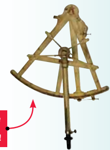
John Bird sextant One of the most important navigational tools ever invented, the sextant (and its ilk) measures the angle between the horizon and an object in the sky to help people determine their geographic location. Sextants are still readily available—and don't require satellites or batteries.
