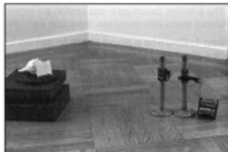
The shoebbox holograph set-up. Laser pen is mounted on the right. A couch shell on the left sits on a motion dampening foundation. A white card is used to focus where the film plate will be.
